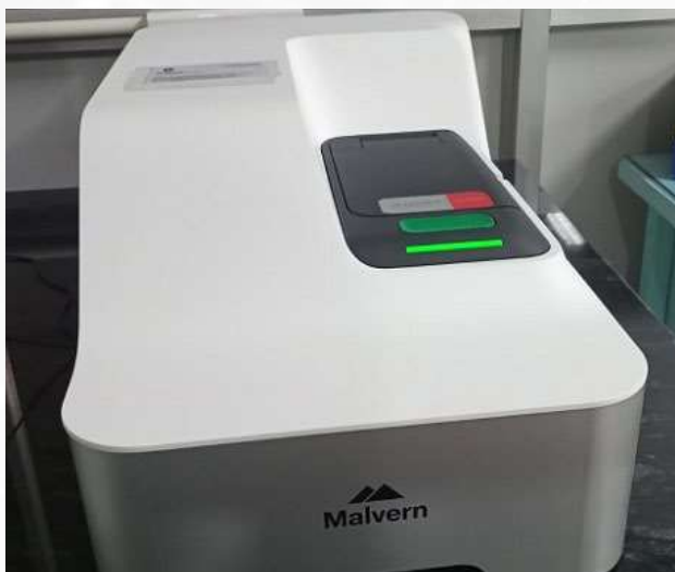
Particle Size and Zeta potential Analyzer, SAIF IIT Patna
