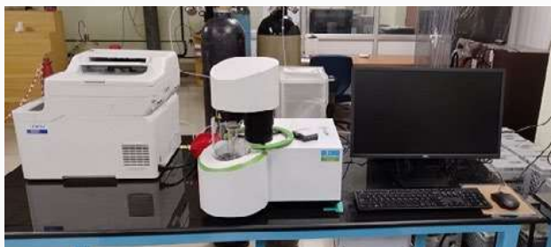
Thermogravimetric Analyzer, SAIF IIT Patna
